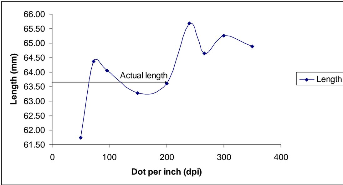
Figure 1. Estimated lengths of a 63.6 mm wire using MSU-RIPL software. Scanned images were made at 9 different dpi resolutions, black and white, and saved as JPEG files before submitting to the website.
