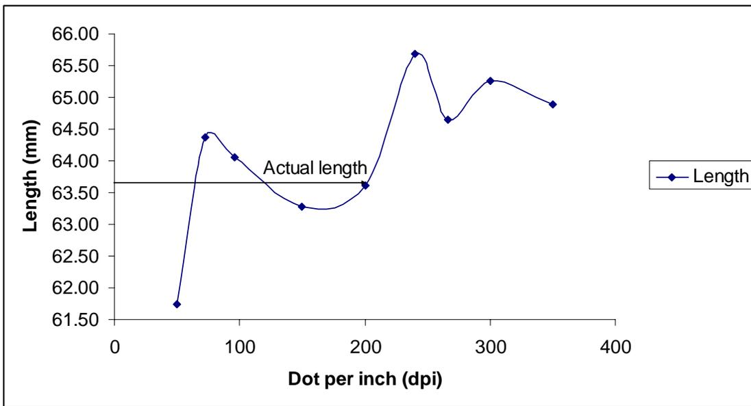
Figure 2. Estimated lengths of a 63.6 mm wire using MSU-RIPL software. Scanned images were made at 9 different dpi resolutions, black and white, and saved as JPEG files before submitting to the MSU-RIPL website. Note that 200 dpi appeared to give the best estimate of actual length. This will change depending upon your scanner.
